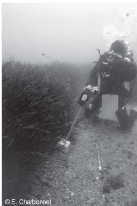
Fig. 153 . Laying a cement marker on the limit of a Posidonia oceanica meadow. The progression, stability or regression of the meadow compared to the cement marker position are then measured. Photo by E. Charbonnel.
