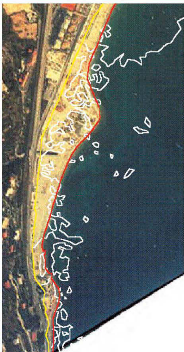
Fig. 68. 1973 aerial photo of the coast between Noli and Spotorno (Liguria, Italy). In yellow, the coastline in 1954, in red the coastline in 1973. From the aerophotogrammetric archives of the Liguria region. Crafted on Mapinfo Professional®. From Maggioncalda (2002).
