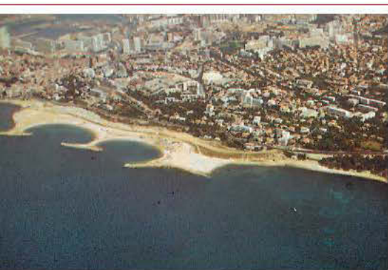
Fig. 57. The artificial beaches of Mourillon (Toulon, Var, France) were built over a Posidonia oceanica meadow, in particular a barrier reef. The most recent development (a nautical club), on the right, does not appear in this photograph. From Astier et al. (1980).
